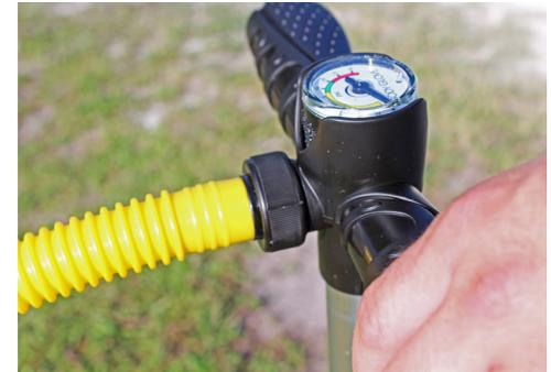
**STEP 5 :** Switch the pump from Single Action (1) to Dual Action (2) for quicker inflation of the platform. In this position the pump pushes air through the hose during both the downward push and the upward pull.
